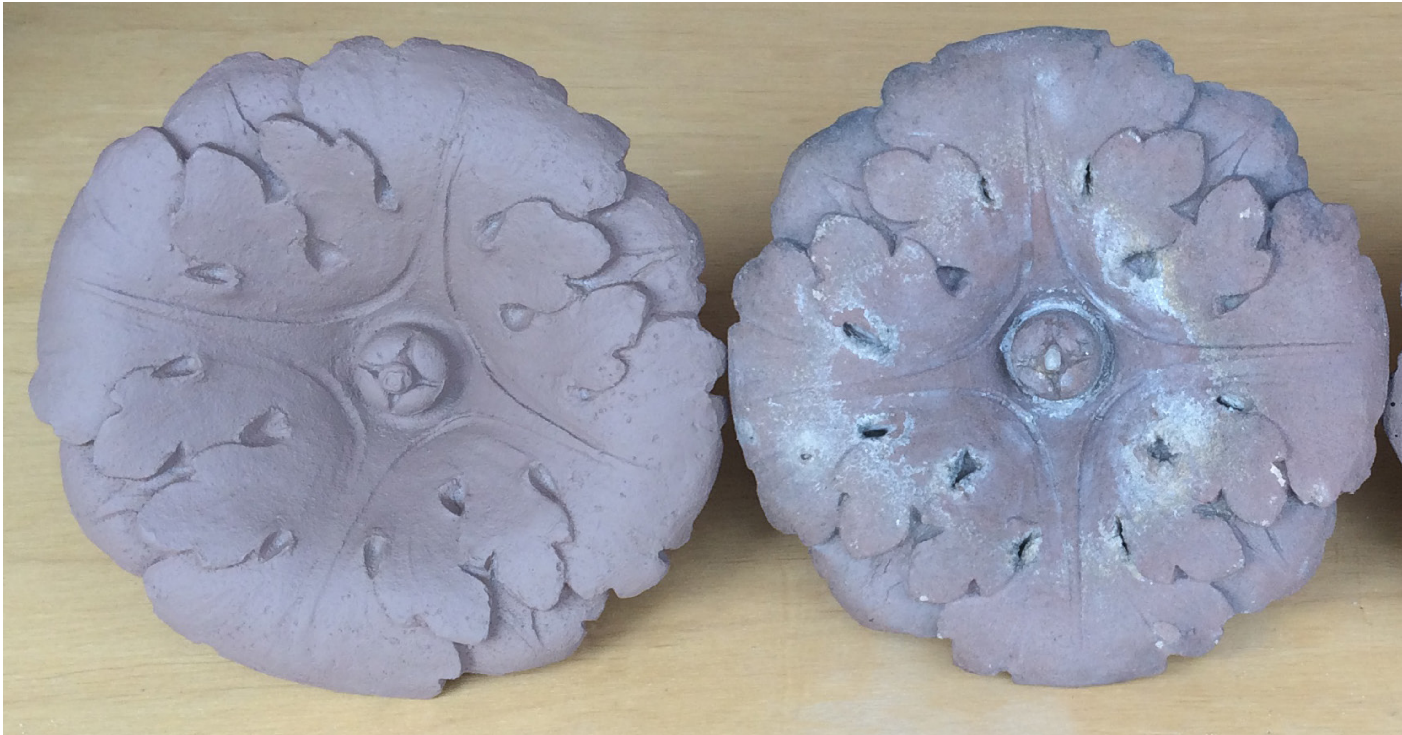
FIBERGLASS REPLACEMENT SAMPLE (LEFT) AND ORIGINAL TERRA COTTA (RIGHT)
