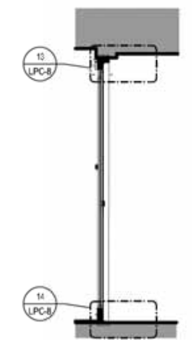
10 EXISTING FRONT DOOR SECTION LPC-12A SCALE: 1/4" = 1'-0"
