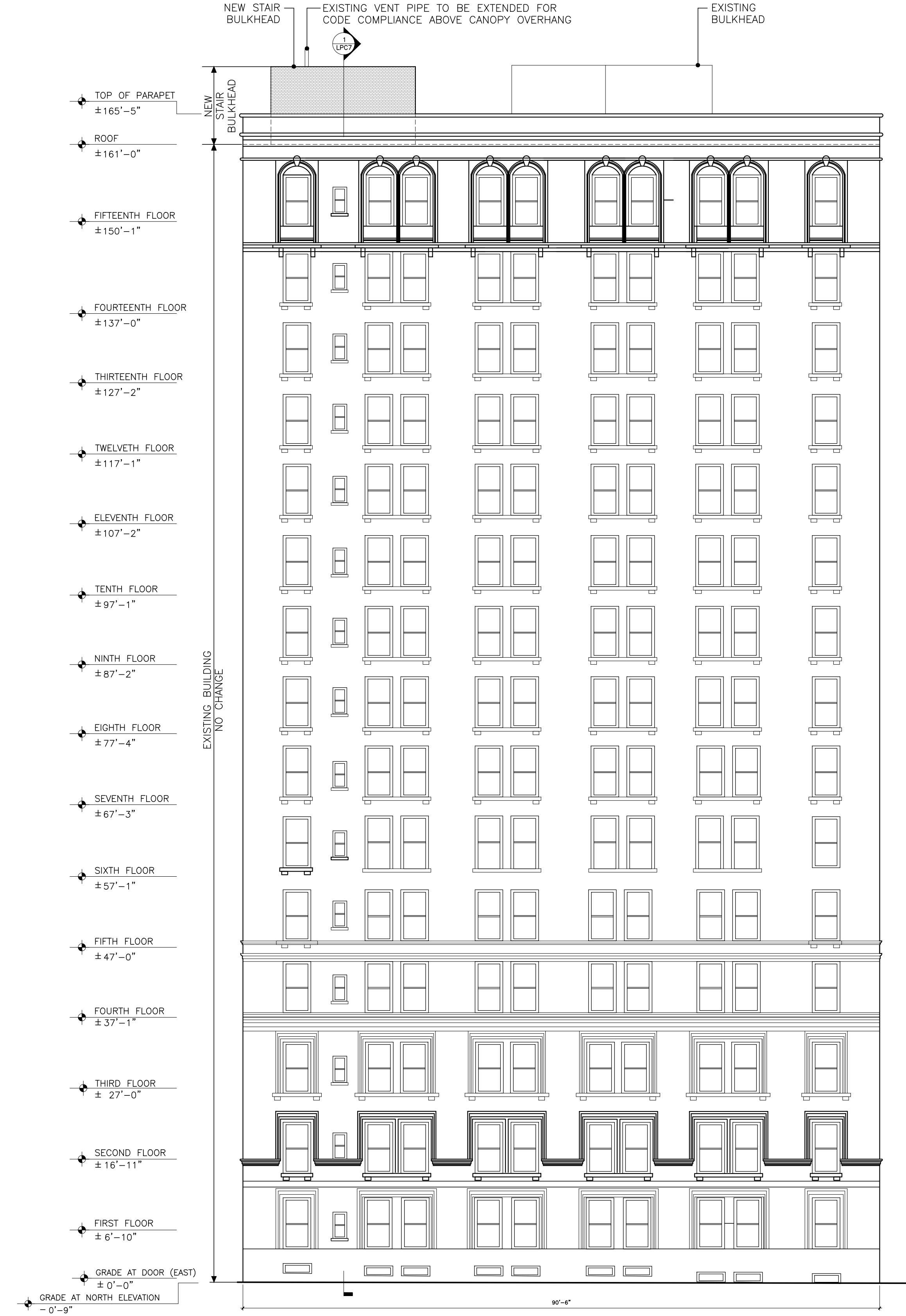
2 PROPOSED NORTH ELEVATION - WEST 83RD ST. SCALE: 3/32" = 1'-0"
