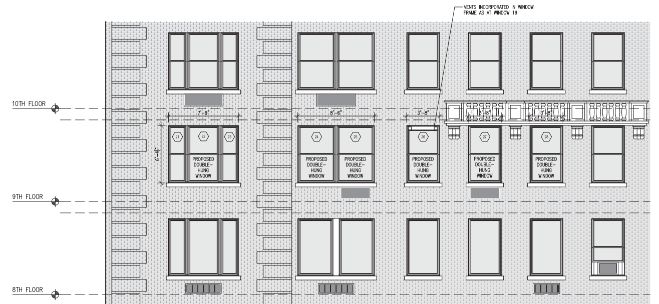
PROPOSED ELEVATION - 87TH STREET 3/16" = 1'-0"
