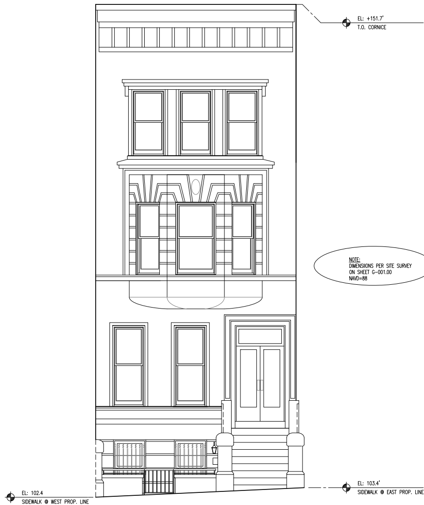
1 FRONT (SOUTH) ELEVATION- EXISTING A-201 1/4"=1'-0"
