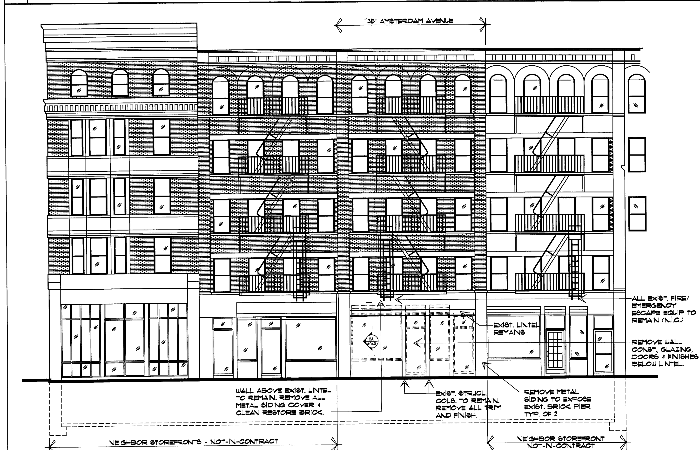
4 FRONT ELEVATION DEMOLITION (AMSTERDAM AVE ELEVATION) 1/8"=1'-0"
