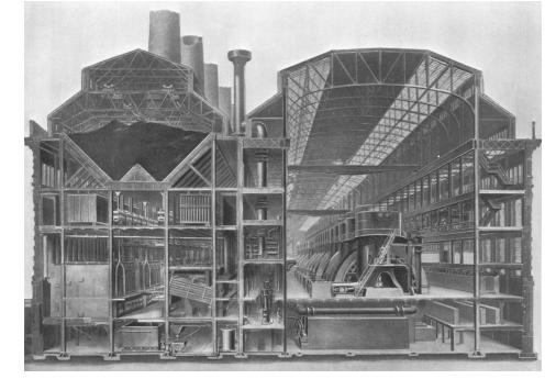
IRT Powerhouse, section drawing showing boiler house (left) and operating room (right), c. 1904 The New York Subway: Its Construction and Equipment, 68.
