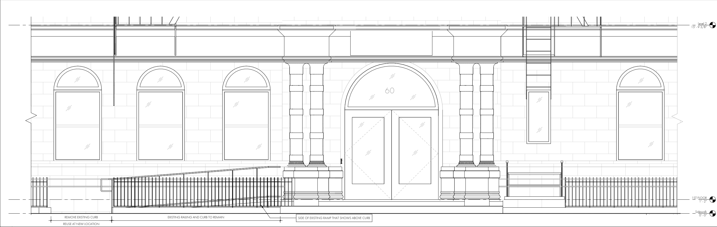
E1 ELEVATION - PROPOSED ENTRANCE 1/2" = 1'-0"
