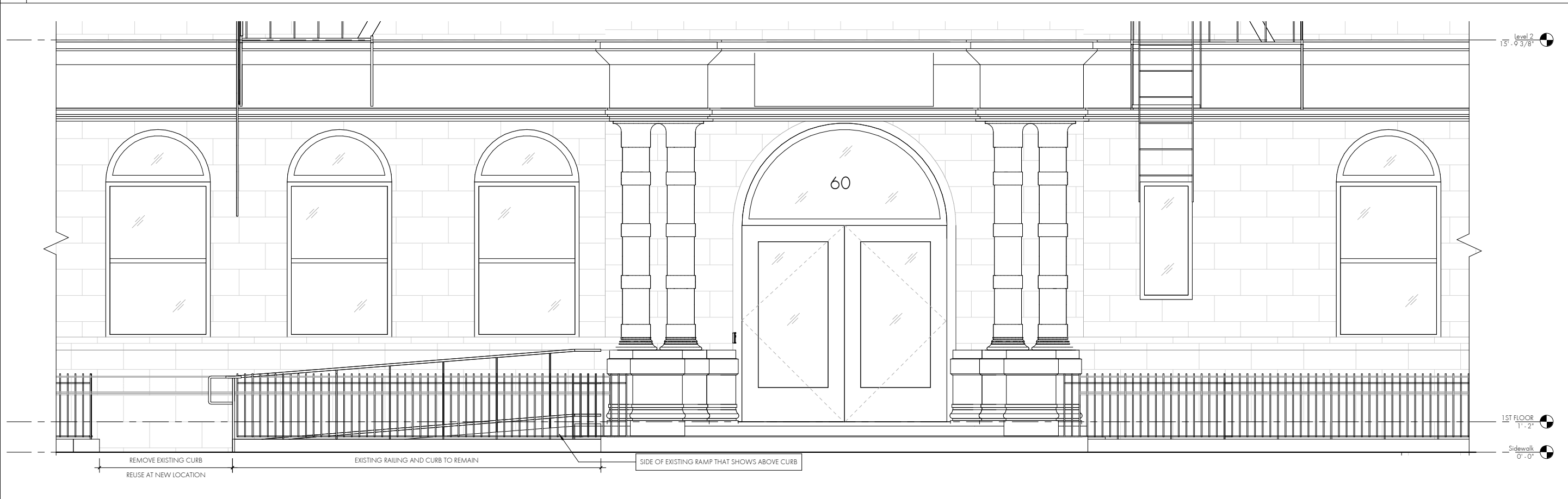
E1 ELEVATION - PROPOSED ENTRANCE - COMMUNITY BOARD RESPONSE 1/2" = 1'-0"
