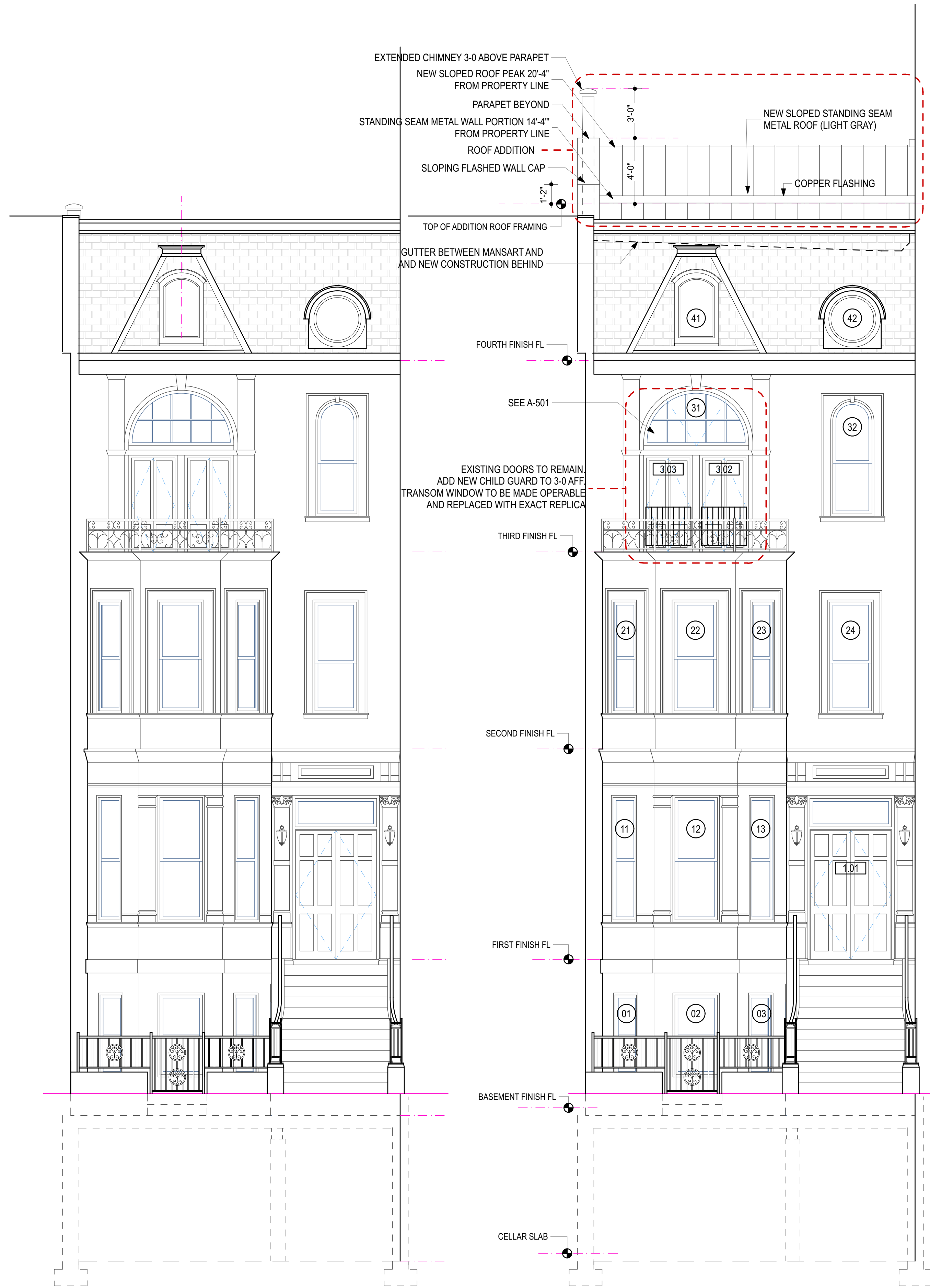
1 EXISTING W 87TH ST (SOUTH) ELEVATION SCALE: 1/4" = 1'-0"
