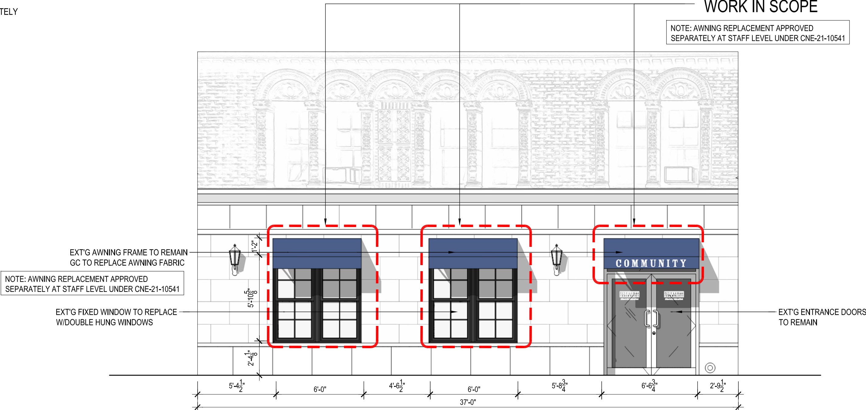
3 PROPOSED STOREFRONT ELEVATION SCALE: 1/4"=1'-0"
