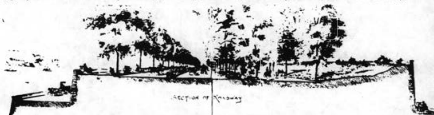
Fig. 10. Peter B. Sweeny, Rotten Row project for Riverside Park, 1890. Sweeny showed the railroad tracks sunk in a deep cut at far right, horse-driving lanes and riding paths on landfill between the tracks, and a commercial lane near river's edge, far left (Sweeny, New York's Greater Rotten Row , 1890).
