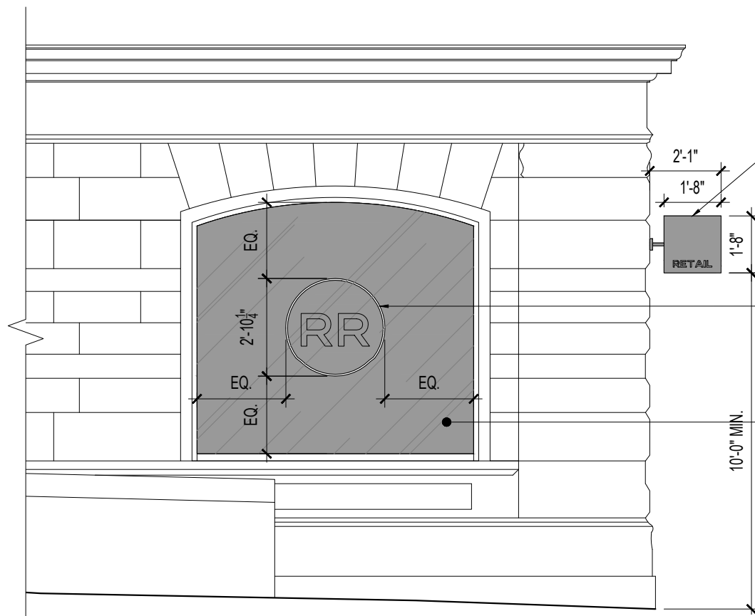
A 69TH ST ELEVATION SCALE: 1/4" = 1'-0"
