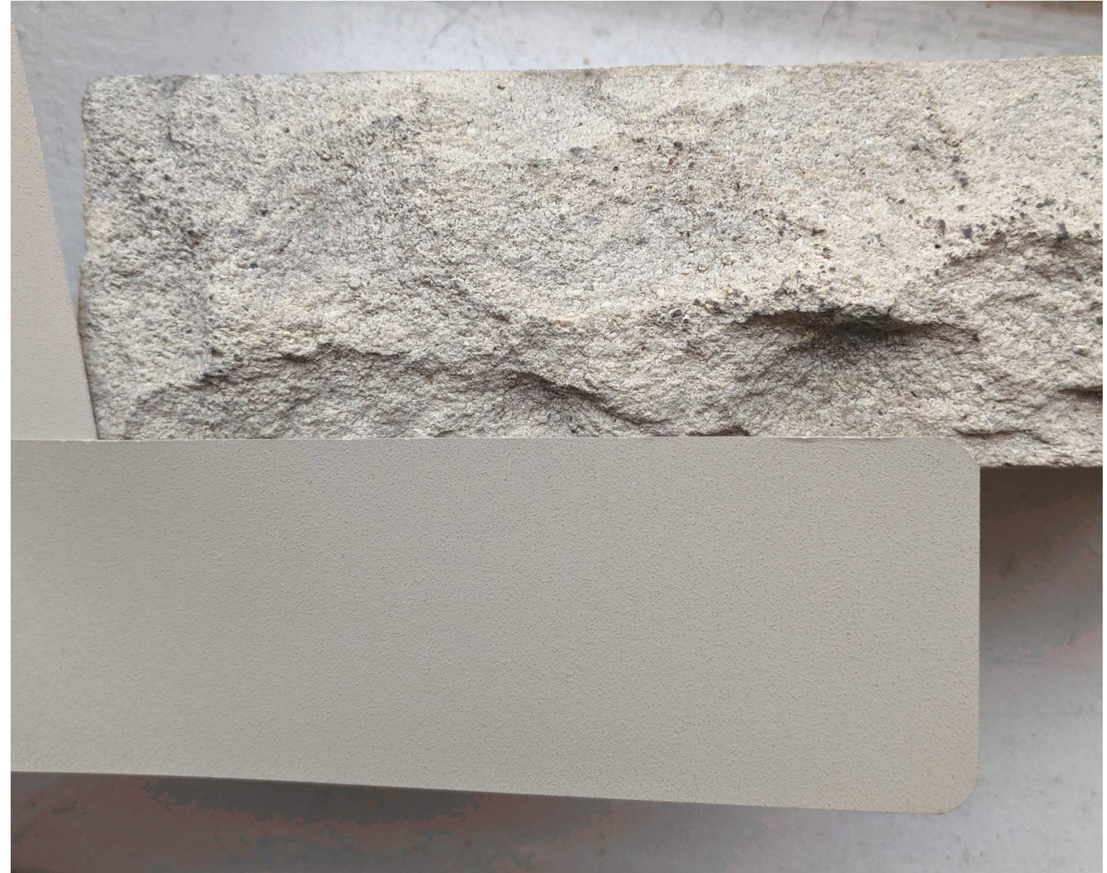
KEIM S117 SWATCH (ALTERNATIVE), SHOWN NEXT TO A REMOVED MAIN FACADE HISTORIC BRICK
