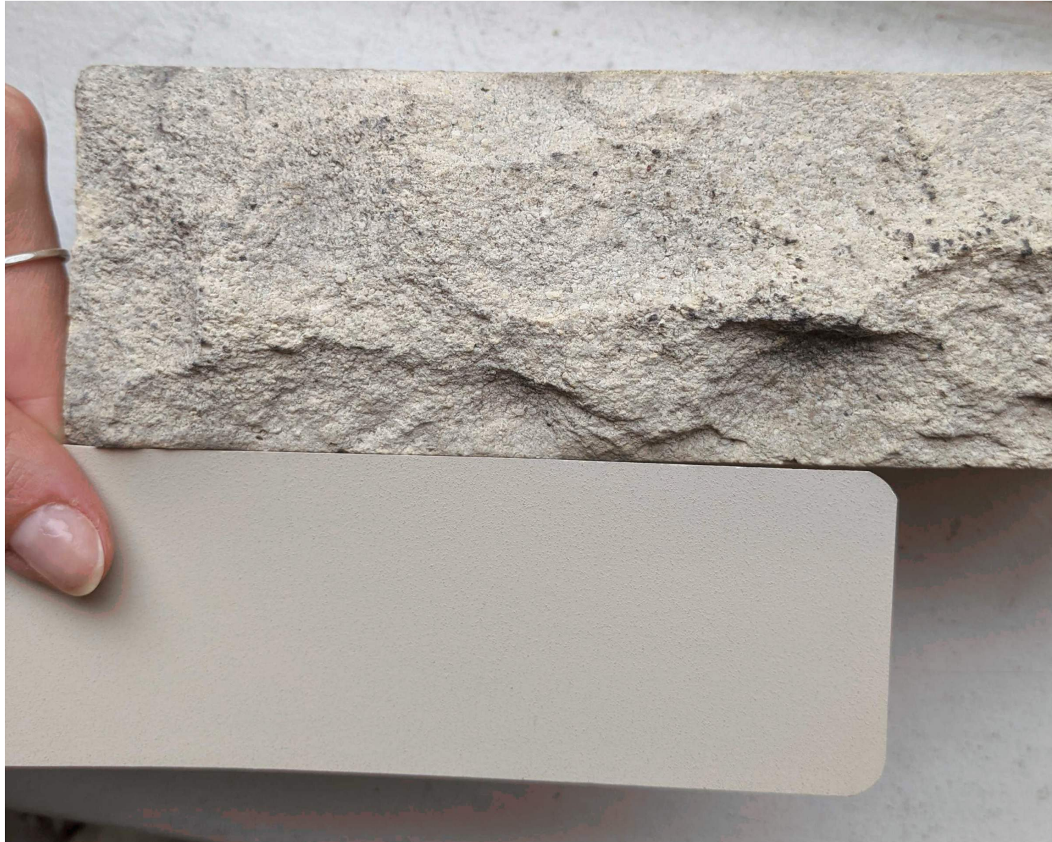
KEIM S119 SWATCH (PREFERRED), SHOWN NEXT TO A REMOVED MAIN FACADE HISTORIC BRICK
