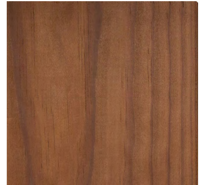
Finish of Picnic Tables and Benches, TYP. Wood Slats: Kebonized Radiata Pine
