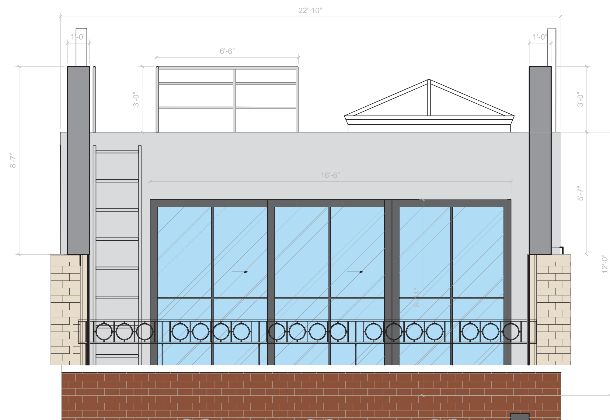
PROPOSED ENLARGED - REAR (NORTH) ELEVATION
